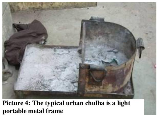
**Picture 4: The typical urban chulha is a light portable metal frame**
